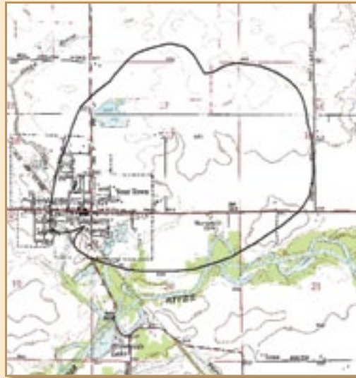
An example of a wellhead protection area, representing the five-year time of travel of ground water to the well.
